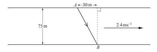
The diagram shows a river with parallel banks. The river is 75 m wide and is flowing with a speed of  $2.4 \,\mathrm{ms^{-1}}$ . A speedboat travels in a straight line from a point A on one bank to a point B on the opposite bank,  $30 \,\mathrm{m}$  downstream from A. The speedboat can travel at a speed of  $4.5 \,\mathrm{ms^{-1}}$  in still water.
